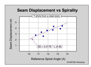
The diagram shows the results of some measurements of seam displacement made on a series of plain jersey T-shirts, compared to those predicted by the simplified equation.
