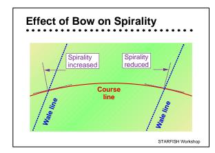
In the simplest case, the angle is positive at the left side of the fabric, decreases to zero at the centre, and then decreases further to negative skew of equal magnitude at the right side.
