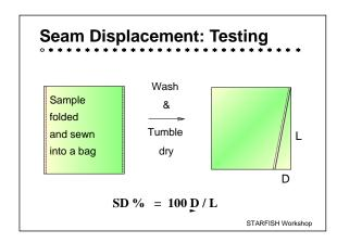
A practical test for seam displacement is carried out by taking a rectangular sample of fabric, whose length is double its width, and sewing it into a bag - a kind of simulated garment.
