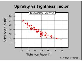
The left hand diagram illustrates the effect of yarn count and stitch length on the reference spiral angle for three yarn counts Ne 20, Ne 32 and Ne 40. The right hand diagram shows the reference spiral angle plotted as a function of the fabric tightness factor for a similar series of fabrics made from Ne16 to Ne 40 yarns.
