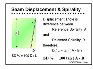
The percentage seam displacement can be related to seam displacement, as described earlier, by means of the following facts.
