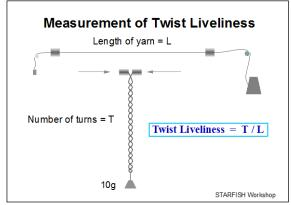
The twist in a singles yarn causes torsional forces to develop in the fibres which tend to make the yarn try to untwist. If a length of singles yarn is held at each end and the ends are slowly brought together, the yarn will twist up upon itself. This effect is called snarling and the torque in the yarn that causes it is called twist liveliness. When the yarn is knitted into a fabric, the consequence of twist liveliness is that the loop twists and bends out of shape. Its twisted shape is such
