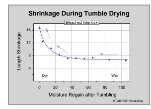
The diagram shows the relationship between shrinkage and moisture content as a fabric dries in a tumble dryer. Shrinkage does not start to take place until the moisture content is below 35% but continues all the way down to about 2% moisture content. Drying cotton to below its natural moisture content (about 7%) is expensive so the finisher sometimes has to choose between maximum relaxation and minimum cost.
