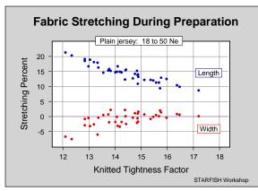
The graph shows some typical results on a wide range of plain single jersey fabrics. It can be seen that the level of distortion is strongly related to the knitted tightness factor. Loosely knitted fabrics are much more extensible than tight ones, and show correspondingly higher levels of distortion after preparation and dyeing.
