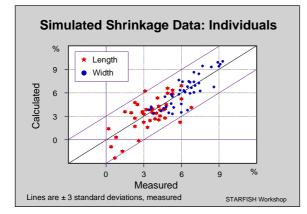
It should be noted that the average standard deviation for the shrinkage testing was about one percentage point. Therefore, we should expect that the average simulated shrinkage values in the table should be within about one percentage point of the measured values, and the individuals in the diagram should be mostly within about two to three percentage points, if the simulation is to be judged successful. It can be seen that this was actually the case.
