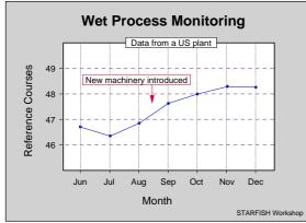
Clearly something happened in the month of August which affected the Reference Dimensions of this normally standard and consistent fabric quality. In fact, the problem coincided with the installation of new machinery with consequent changes in processing routes.
