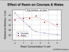
With the interlock construction, the most noticeable effects were in the length direction. The number of courses in the Reference State was reduced in line with the increase in the level of crosslinking chemicals applied.
