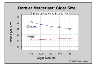
In a trial that was carried out on a Dornier machine, identical pieces of rib and single jersey fabric were processed through the machine using different width settings for the cigar (stretching frame).
