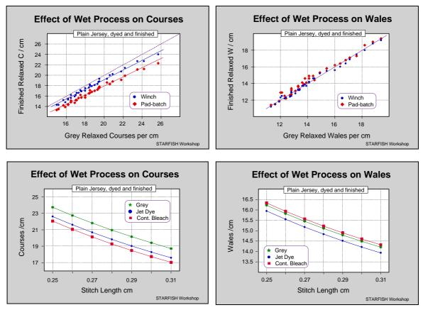
The net result is that the shape, which the loop will obtain in the Reference State, is permanently altered by the Wet Processing. This is reflected in the Course / Wale Ratio.
