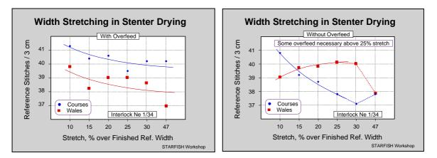
It was found that stretching the fabric from about 10% to 47% over finished reference width caused a small reduction in reference courses when the samples were dried with overfeed. This effect was much larger - especially at high levels of stretching - on the samples dried without overfeed.
