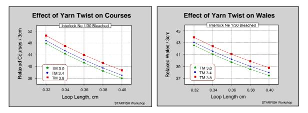
The same is also true for rotor spun yarns. Yarns spun with a higher twist multiple will develop more courses and wales in the fabric in the Reference State than yarns spun with a lower twist multiple.
