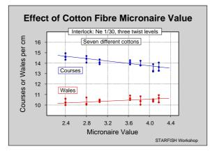
Dimensions. A set of OE rotor yarns were spun from a group of seven cottons with widely different Micronaire Values, each spun to the same yarn count at three levels of twist, and all knitted into interlock fabrics with approximately the same stitch lengths.
