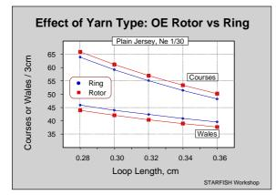
the Reference State compared to an equivalent fabric knitted at the same stitch length and yarn count but produced from ring spun yarn.
