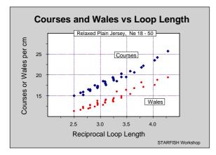
For a given yarn quality, the average stitch length determines the number of courses and wales which will be developed in a fabric in its Reference State of Relaxation. The course and wale densities determine the length, width and weight of the fabric.
