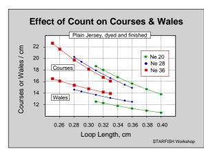
and weight of the knitted loop. A coarser (heavier) yarn, knitted at the same average stitch length and finished to the same dimensions (course density and width) will produce a heavier fabric than if the same fabric had been produced from a finer (lighter) yarn.
