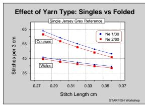
Reference State compared to an equivalent fabric knitted at the same stitch length and yarn count but produced from a singles yarn.
